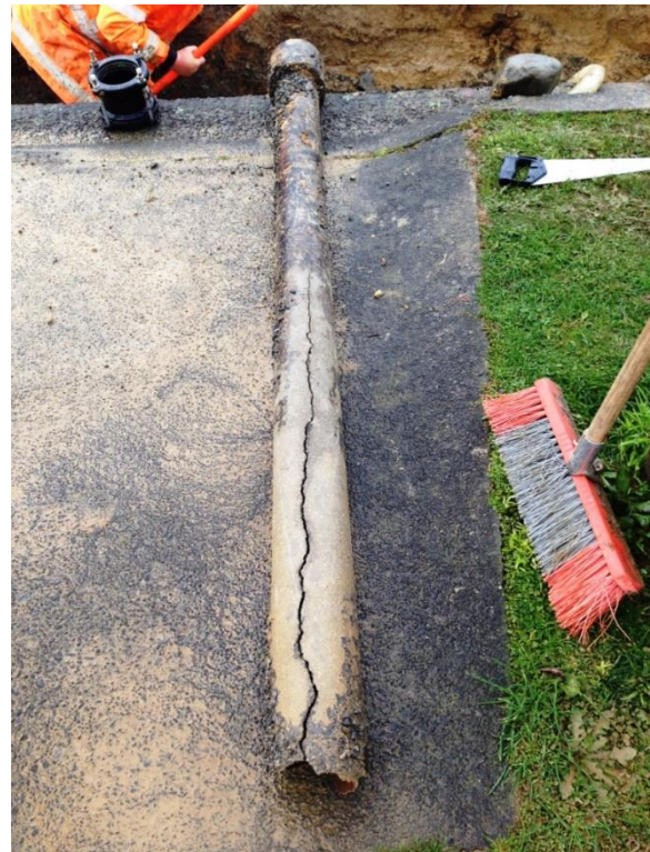
Existing 100mm diameter asbestos cement pipe showing a large longitudinal crack; proof that the old pipe has reached its end of life.
