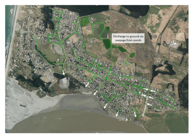
The discharge points are shown in the diagram above. There are five discharges direct to the Estuary, some seepage to ground through the attenuation ponds, and some discharges direct to Whitebait Creek.
